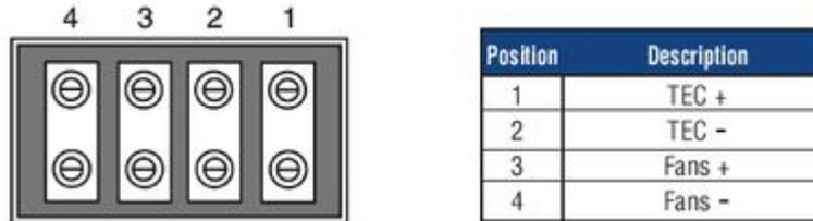
Figure 1- Power Connector of MPA075-12 ([www.lairdtech.com](http://www.lairdtech.com))
