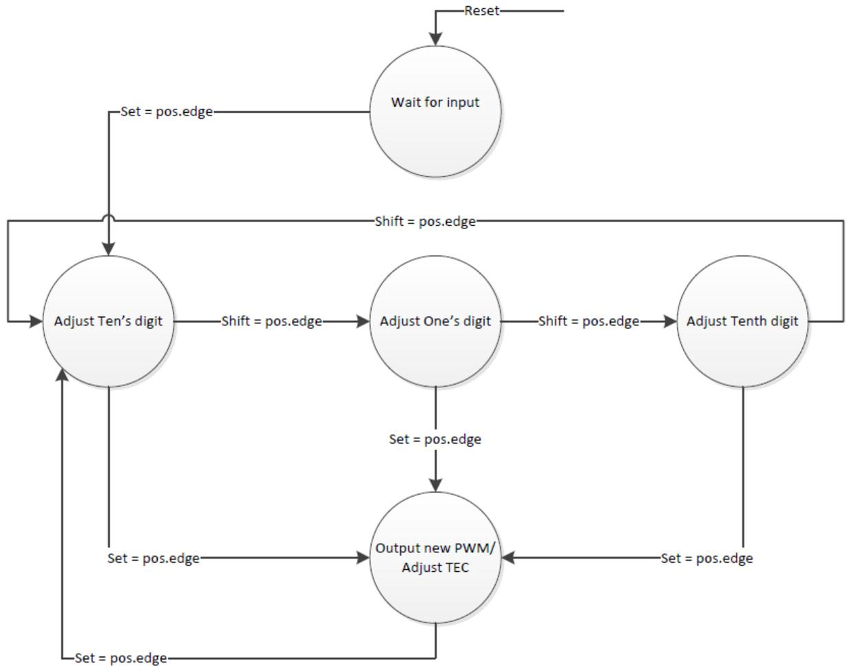
Figure 3 - FSM diagram of Temperature Controller
