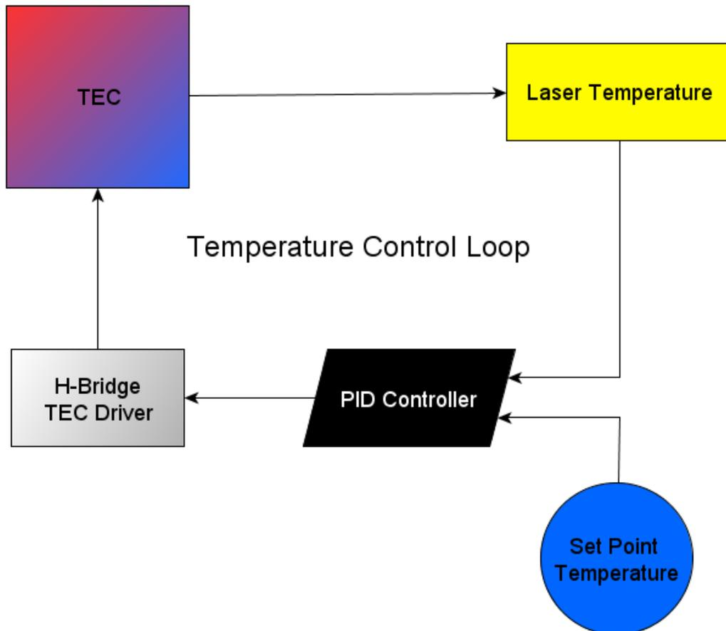
Figure 4 - Temperature Control Loop
