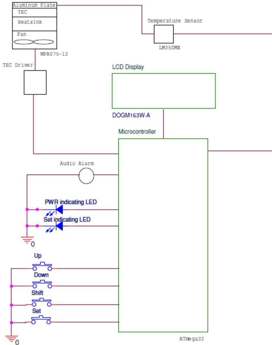
Figure 6 - A high-level block diagram showing the major components of the system
