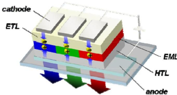
Figure 2. OLED Structure, ETL (Electron Transport Layer), EML (Emitter Layer, HTL (Hole Transport Layer)
